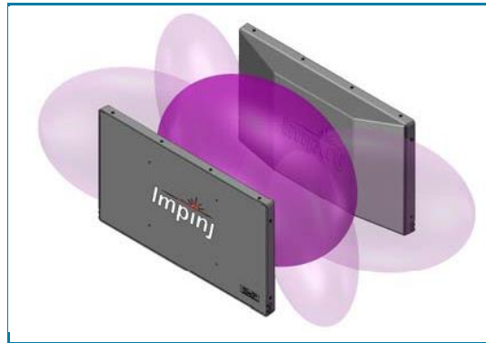
Figure 2: Guardwall Read Zone Diagram
